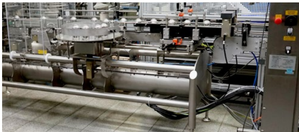
The chain checkweigher offers maximum stability for most accurate weighing results.
