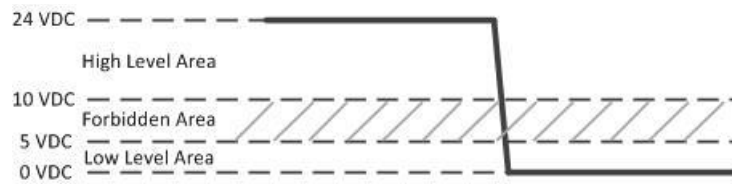
Figure 3-11: A Falling-edge Trigger Signal on Input
