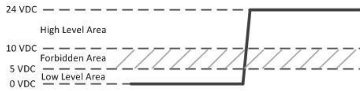
Figure 3-10: A Rising-edge Trigger Signal on Input
