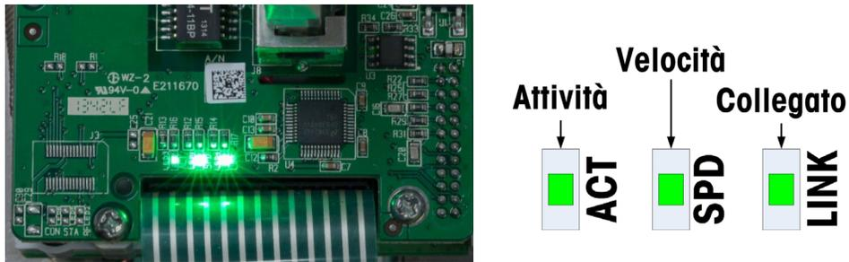
**Figura 5-10: LED Ethernet TCP/IP**
